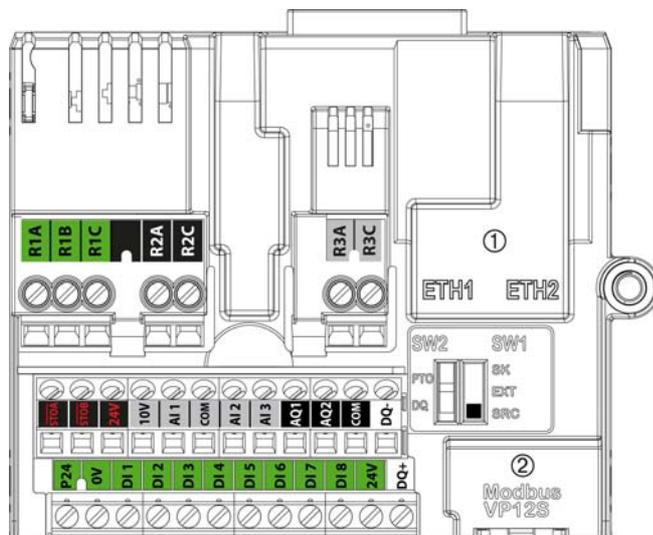
① Ethernet Modbus TCP, ② Serial Modbus
